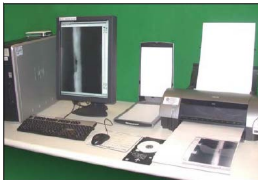
Typical NDE Workstation with 3MP Monitor
