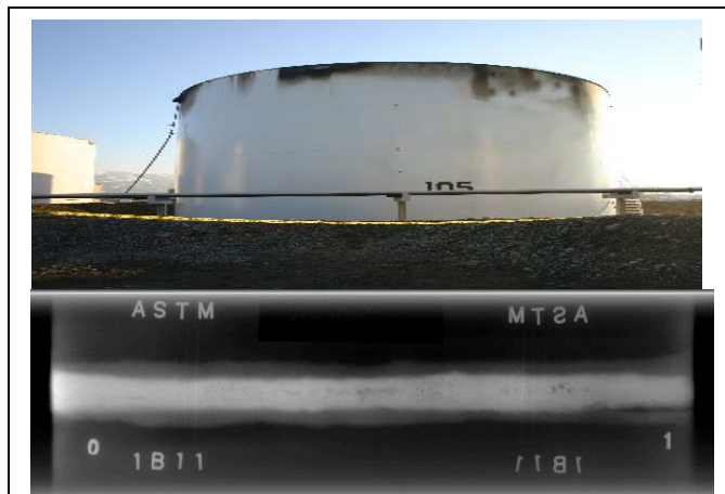
Storage Tank Weld Radiography Image
